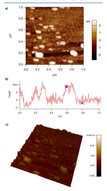
**Figure 2.** (a) AFM  $(1 \times 1 \ \mu m)$  topography image of nanoparticles **NP1** casted on a polyethylenimine (PEI)-coated Si wafer. (b) The *z*-profile across the red line of the 2D AFM image in (a). (c) 3D height mode AFM  $(1 \times 1 \ \mu m)$  image of the nanoparticles in (a).
